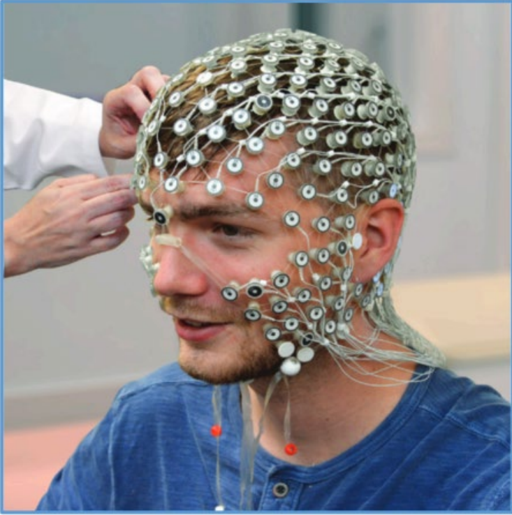
Figure 2. Whole head sensor net distribution of 256 electrodes.
